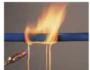
Other Plastics - initially when torch is applied
