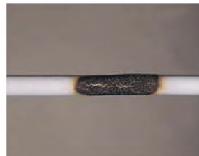
CPVC - After torch is removed
