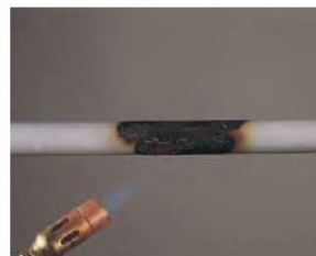
CPVC - initially when torch is applied
